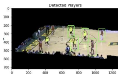
Figure 5: Players detected using Hog pedestrian detection
