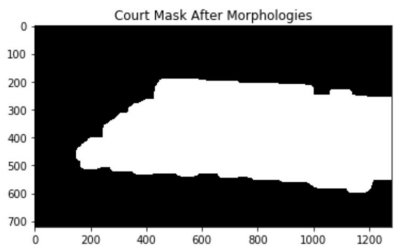
Figure 3: Erode and dilate filters applied to remove artifacts
